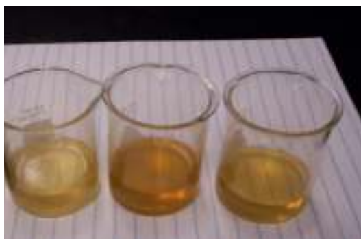
L-R, 1.0 mM microwaved alginate, 1.0 mM boiled alginate and 2.0 mM microwaved alginate.
