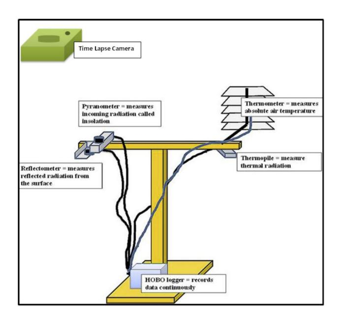
Figure 2: Our experimental setup.
