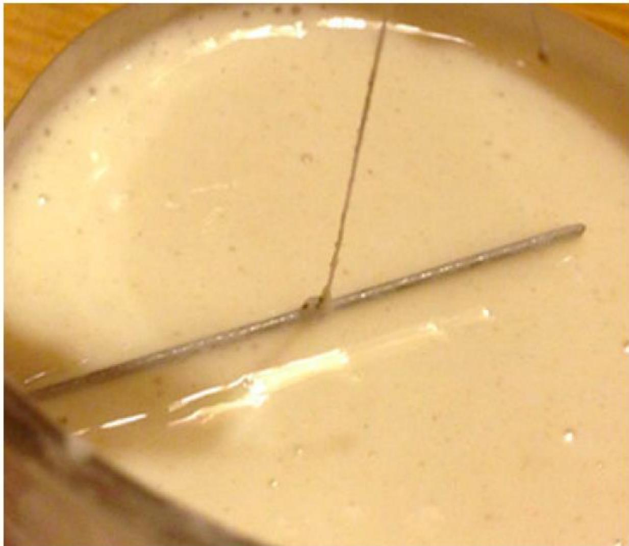
Figure 4: Surface tension. Just before the flour solution released the needle, the surface tension appeared to be “pulling” it.
